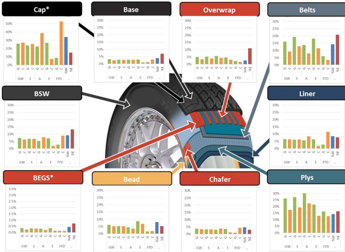
Figure 22. Normalized Guayule (green) and Hevea (orange) Tire Component Impact Comparison. The results include only the manufacturing impacts of the raw materials comprising the components; this includes the agricultural and processing inputs for guayule and Hevea. Raw material transport and tire manufacturing electricity are not included. Components' % Weight in Tire (blue), and % Manufacturing Electricity Consumption (red). *Note that the scale in impact graphs for these parts has been altered for ease of display. Abbreviations: GW – Global Warming; S – Smog; A – Acidification; E – Eutrophication; FFD – Fossil Fuel Depletion; %W – the mass portion of the particular component in relation to the total mass of tire components; %E – the portion of electricity consumed in the manufacturing of the particular part in relation to the total electricity consumed for component manufacturing.
