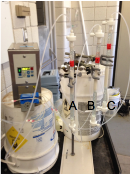
Figure 3.14: Passive Samplers Setup at Chandler WTP
