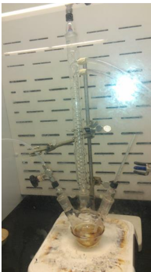
Figure 32. Ionic liquid synthesis setup
