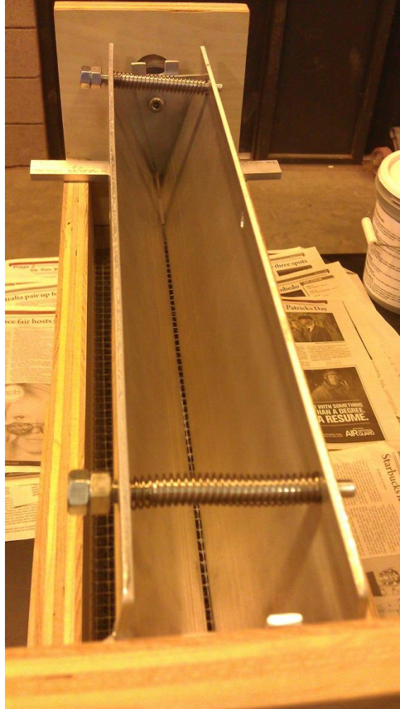
Figure 3-5: Fabricated Bead Dropper
