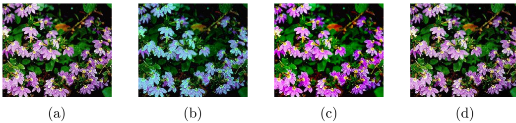
Figure 4.4: Examples of color transformations: (a) Original texture; (b) Hue transform; (c) Saturation transform; (d) Contrast transform.
