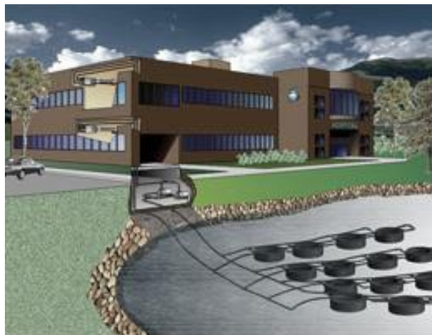
Figure 1.11: Surface Water Closed Loop (Mammoth, CES group)
