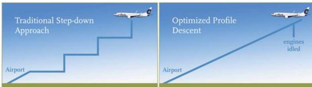
Figure 9. Traditional Step-Down Approach vs. Continuous Descent Approach
