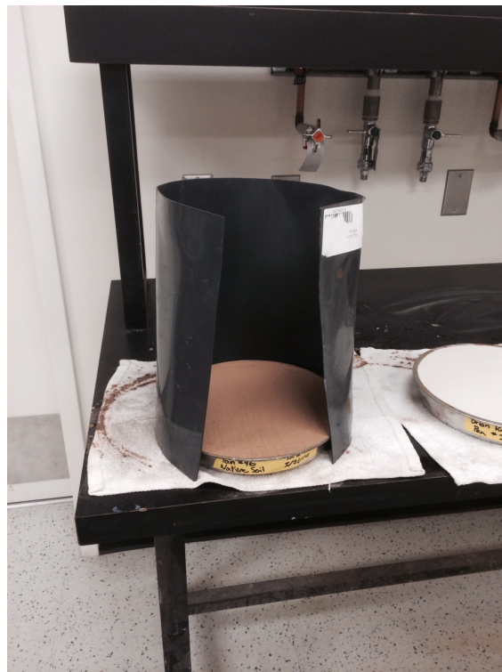
Figure 21: Native Soil Pan Prior to Spray Application
