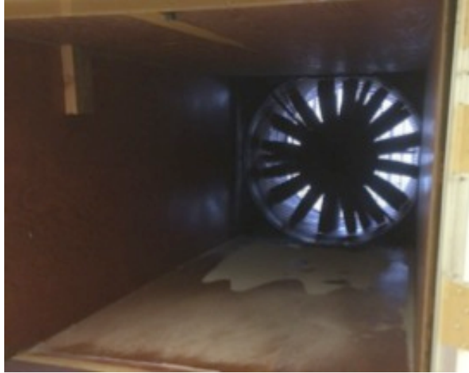
Figure 12: Rear Fan of Wind Tunnel.
