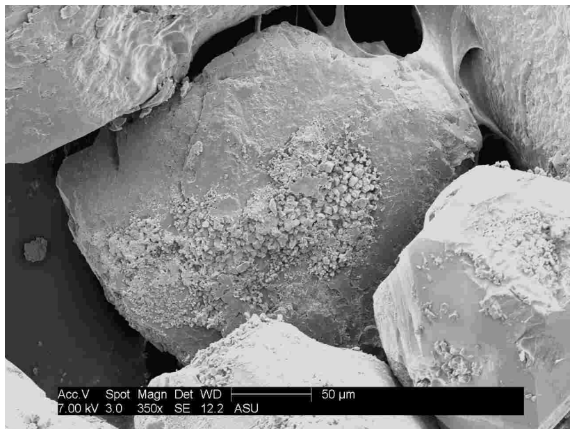
Figure 36: SEM Image of F60 particle with carbonate precipitation
