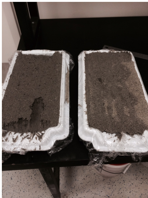
Figure 42: Water Erosion test Specimens Compared after 3 Minutes of Water Flow
