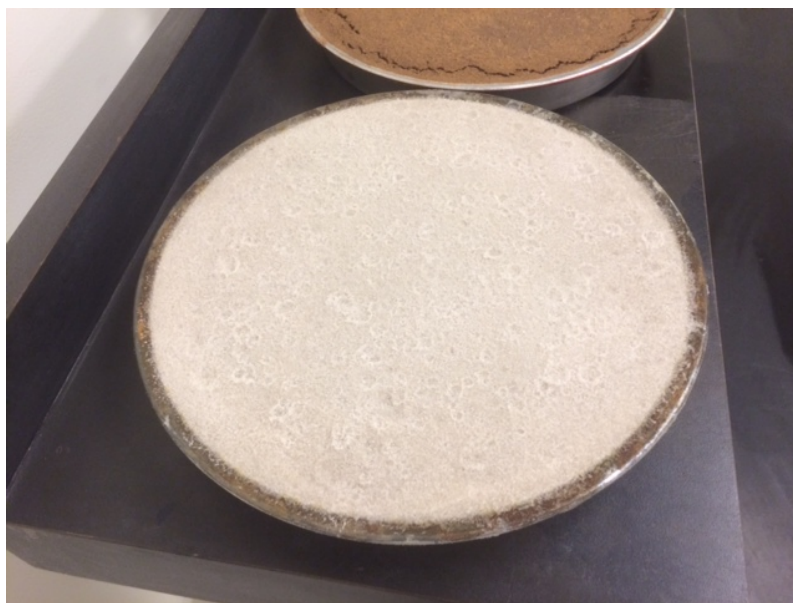
Figure 14: F60 soil pan sprayed with \text{CaCl}_2 and Urease Solutions
