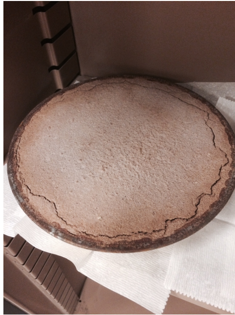
Figure 24: Native Soil Pan Turned White from Carbonate
