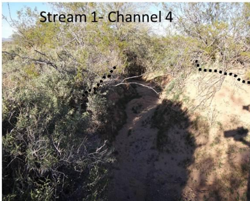
Figure 19. The above aerial photograph displays the channels that were surveyed in the field to calculate bankfull discharge rates. Stream 1 had eight channels (numbered in the aerial photo above) and Stream 2 had one channel. The photographs are examples of channel characteristics of the two sites where the dotted black line denotes the bank.
