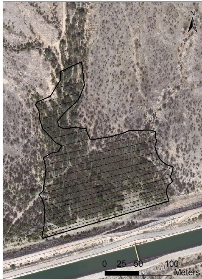
Figure 21. The figure displays the 20 transects used to calculate the total average volume contained in the green-up zone when flooded. The black boundary signifies the green-up zone boundary.
