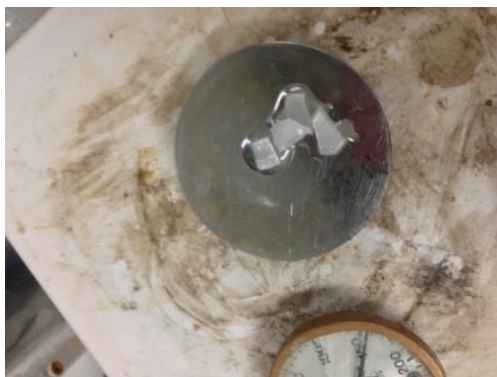
Figure B.5. Melting pieces of water soluble Crystalbond™ (wax like)
