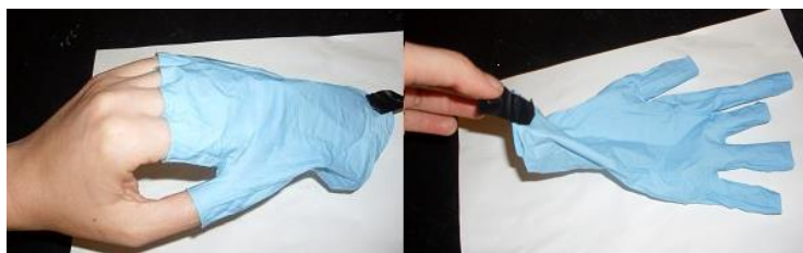
Figure C.2. Removal of the gloves using the tab. Notice that after the removal the glove is inside out.
