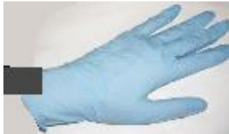
Figure C.1. Gloves with duct tape. Notice that the tab is big enough to remove afterwards the glove without touching the actual gloves.
