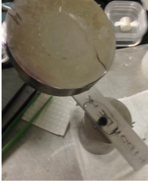
Figure B.6. Pouring molten water-soluble Crystalbond™ (wax like) into the sample.
