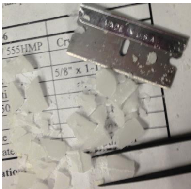
Figure B.4. Sliced pieces of water soluble Crystalbond™ (wax like).
