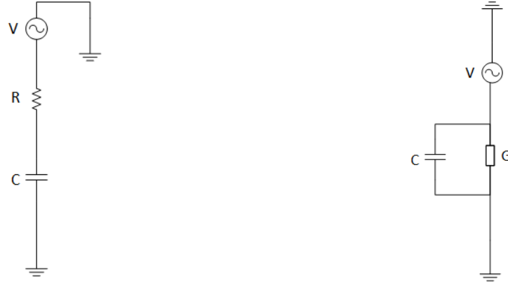
Figure 70. The equivalent circuit for the DUT as seen by the LCR meter in series (left) and parallel (right) modes.
