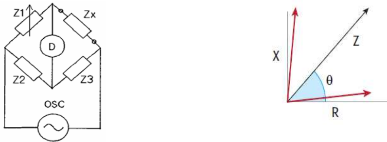
Figure 69. (Left) Bridge circuit in the LCR meter. (Right) phase diagram between the resistance and reactance of the device as seen by the capacitance meter.
