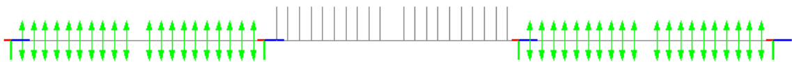
Figure 17. Active people and passive people configuration for an excitation frequency of 2.30 Hz that gives maximum response
