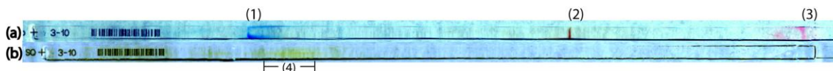
Figure B-2. IEF of protein standard and polyclonal IgG protein. (a) The IPG strip contains IEF isoelectric point (pI) protein standards: (1) phycocyanin (pI 4.45, 4.65, 4.75), (2) myoglobin (6.8, 7.0) and (3) cytochrome c (9.6). (b) The IPG strip of fluorescently labeled Alexa488-IgG.
