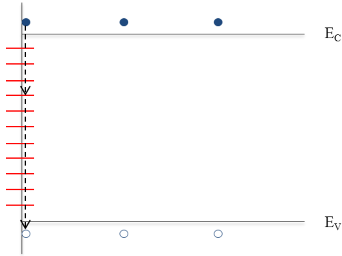
Fig. 2.8. Energy band diagram illustrating recombination via surface states.
