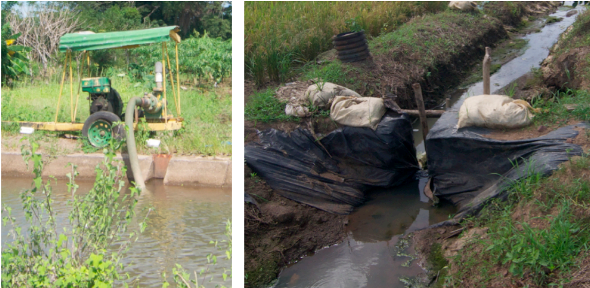
Figure 4.2 – The picture on the left is of a pump illegally drawing irrigation water from a PRAT canal; when water managers are not patrolling the canals, farmers can use pumps to transport water from the canals to their crops during the cycling process, and this limits water availability downstream. The picture on the right is of a makeshift dam, built by a farmer in a remote region of the irrigation district (an area that is infrequently patrolled). Farmers build these dams to gain access to water, and their neighbors typically destroy them as they are affected by the water loss.
