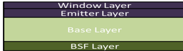
Fig. 2.8 The conventional structure of GaAs solar cells
