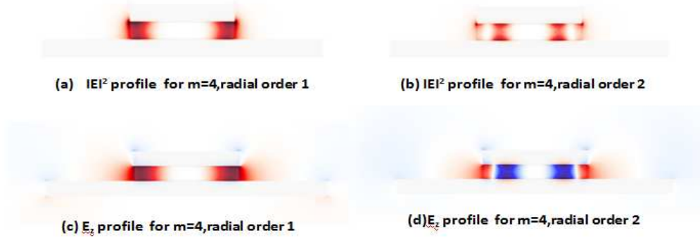
Fig3.3 Field intensity and z component of electric field for WG plasmonic mode ( m=4 )
