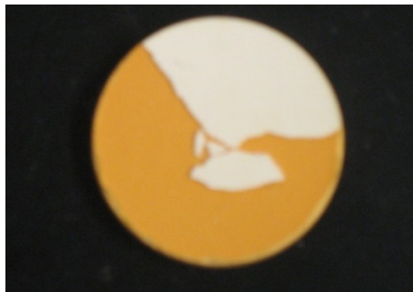
Figure 5.10 Image of thin SDC-carbonate dual-phase membrane peeled from BYS support after infiltration
