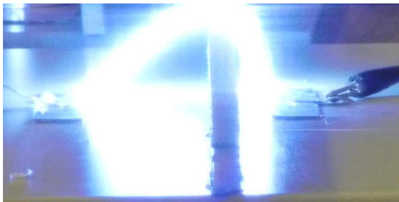
(c) L = 10\text{ cm} , a/L = 0.2 , 2 inch barrier
