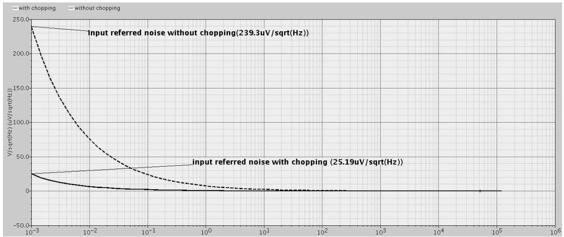
Figure 5.5: Input referred noise of the folded cascode amplifier. Chopping reduces the input referred noise to 25 \mu\text{V}/\text{Hz}^{1/2}
