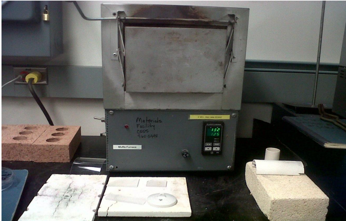
Fig 2.1 Muffle furnace used for the heat-treatment of the carbon composite cores
