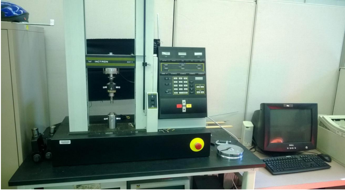
Fig 5.5 The INSTRON 4411 MTS system interfaced to a personal computer
