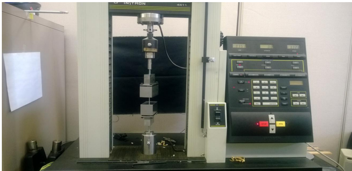
Fig 5.7 Specimen loaded at 5 kN with the help of the custom gripping fixtures on the test frame
