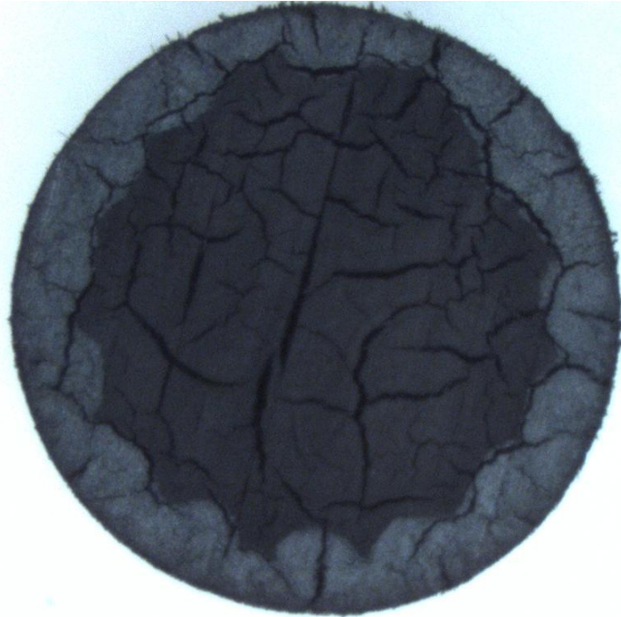
Fig 2.7 Cross section of the sample heat – treated at 300°C for 24 hours
