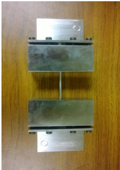
Fig 5.3 ACCR core strand sample held by the custom grips
