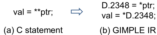
Figure 5.3: One example of the transformation from C code to GIMPLE IR by using our modified compiler
