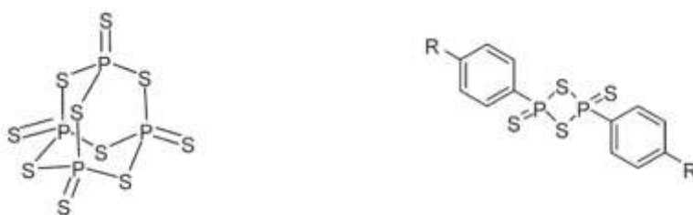
Figure 10. Molecular structures of P_4S_{10} (left) and Lawesson's reagent (right).
