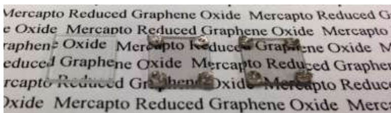
Figure 43. Digital camera photograph of plain glass (left), 92% optical transparent m-RGOs LB film (middle), and 91% optical transparent m-RGOs LB film (right).
