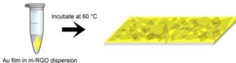
Figure 48. Schematic illustration of deposition of m-RGOs on gold substrate.
