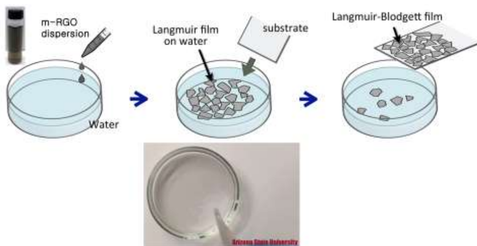
Figure 40. Schematic illustration of m-RGOs LB film fabrication procedure and photographs of m-RGOs dispersion in ethanol and m-RGOs Langmuir film on the surface of water.
