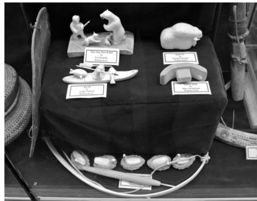
Fig. 427. Ivory drill bow and drill (bottom) with mouthpiece (top right) made by Mike Saclamana of King Island on display inside the Sitnasuak Native Corporation. Nome, AK. 2012.
