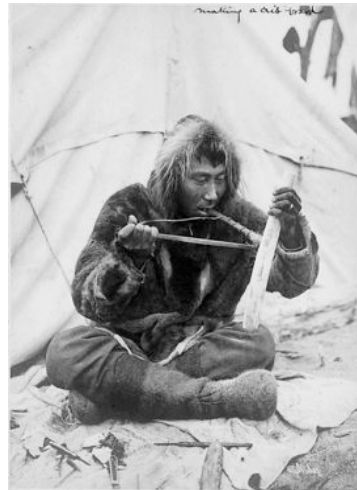
Fig. 300. Alaska Natives at Port Clarence making souvenirs. The drill bow carver is using uses an ivory bow with a scalloped edge similar to those from Point Barrow. Photograph by Eric A. Hegg, 1900. University of Washington Libraries, Special Collections Division, PH Coll 274.
