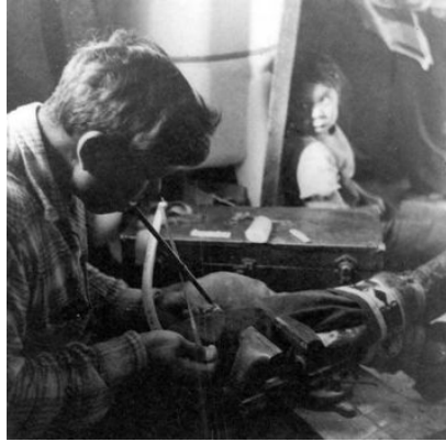
Fig. 30. Charlie Ayapana carving ivory with a bow drill while a child observes from around the corner. Point Hope, AK. 1953-58. Archives, University of Alaska, Fairbanks, UAF-2001-129-56.
