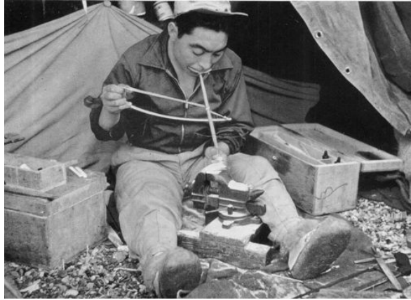
Fig. 38. Oscar Ahkanza from Little Diomed carving ivory with a bow drill on the beach in Kotzebue. Photograph by Amos Burg with the caption “In summer, Oscar sails to Kotzebue to fish, trade, and carve walrus tusks into cribbage boards, boxes, cigarette holders, bracelets and umbrella handles.” (from Burg 1952:68).
