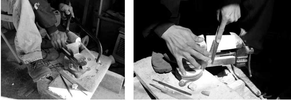
Fig. 418a-b. Gary Sockpick carving ivory in Shishmaref, AK. 2012. a. sawing tusk to create a flat surface. b. sanding ivory while secured in a vise.
