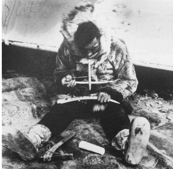
Fig. 14. A bow drill carver in Barrow creating holes for an ivory cribbage board. An unworked section of tusk and an adze are at the carver's feet. Photograph by T. P. Brower, c. 1910 (from Pearce 1985:15).
