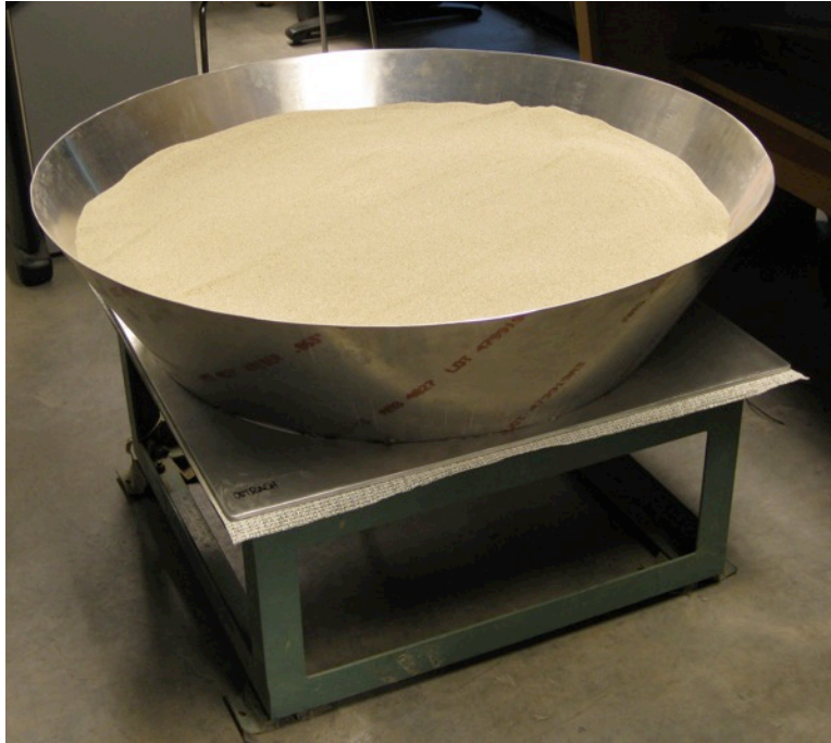
Figure 5.7. Large vertical shaker (Syntron Jogger VP-181) experimental setup, with the custom-built circular pan (base diameter 71.1 cm, top diameter 91.1 cm) filled to ~15 cm depth with sand (300–600 \mu\text{m} size fraction). A rubber non-skid carpet pad was placed between the shaker and the container to minimize movement of the pan during shaking. A tripod was stationed to the lower left of the shaker table (out of the field of view) to which the camera was attached.
