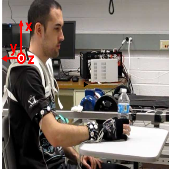
Figure 3.5: Experimental setup: The subjects were seated on a chair with a distance avoiding a full stretch of the arm. An active motion capture system was placed on the right side of the subjects. Position tracking sensors were put on the subjects' shoulder, upper arm, forearm and palm.
