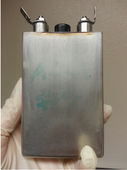
Fig. 2.7 Group I. Ni-Cd battery 2V, 8Ah
