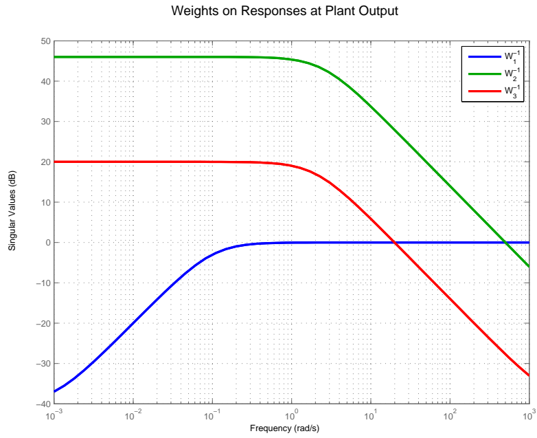
Figure 5.3: Weighting functions output due to reference command
