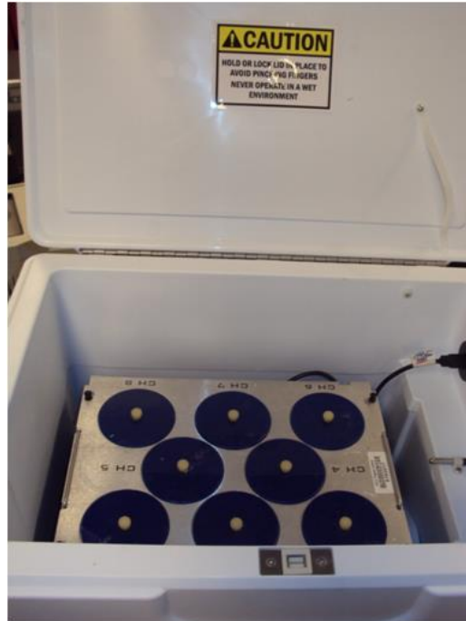
Figure 7: Calmetrix ICal 8000 Isothermal Calorimeter
