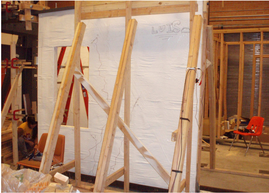
Figure 26. The CarbonFlex-wrapped wall with opening.
