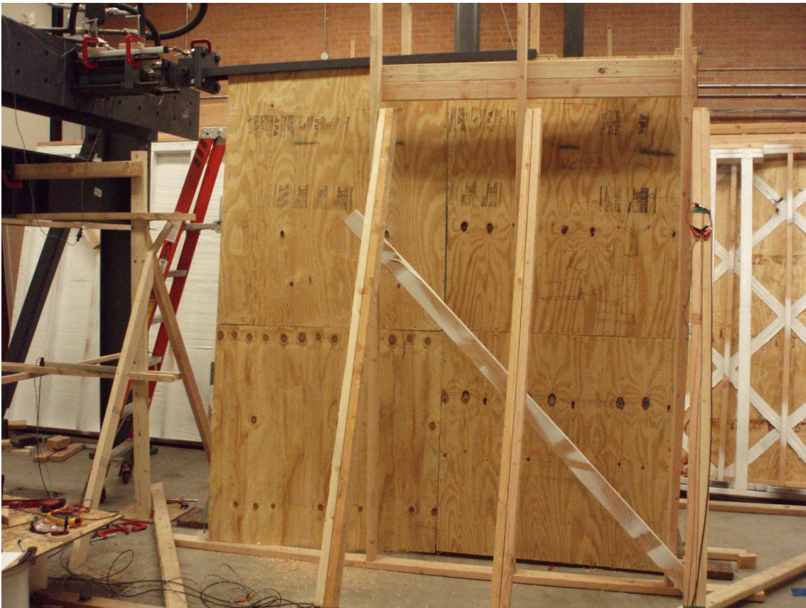
Figure 21. The plywood shear wall number one.
