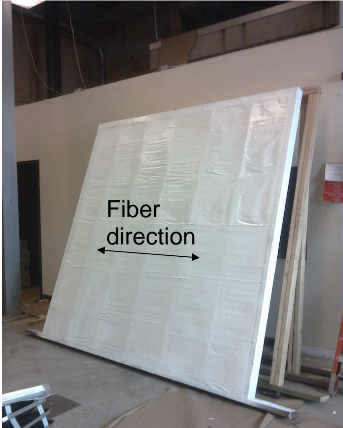
Figure 23. The CarbonFlex fully wrapped wall number one.
