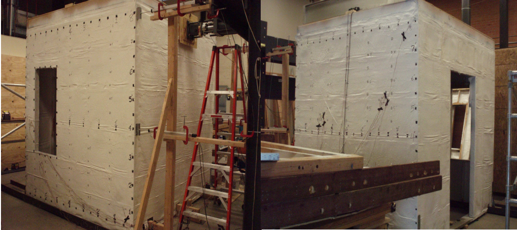
Figure 28. The single-story CarbonFlex-wrapped structure.
