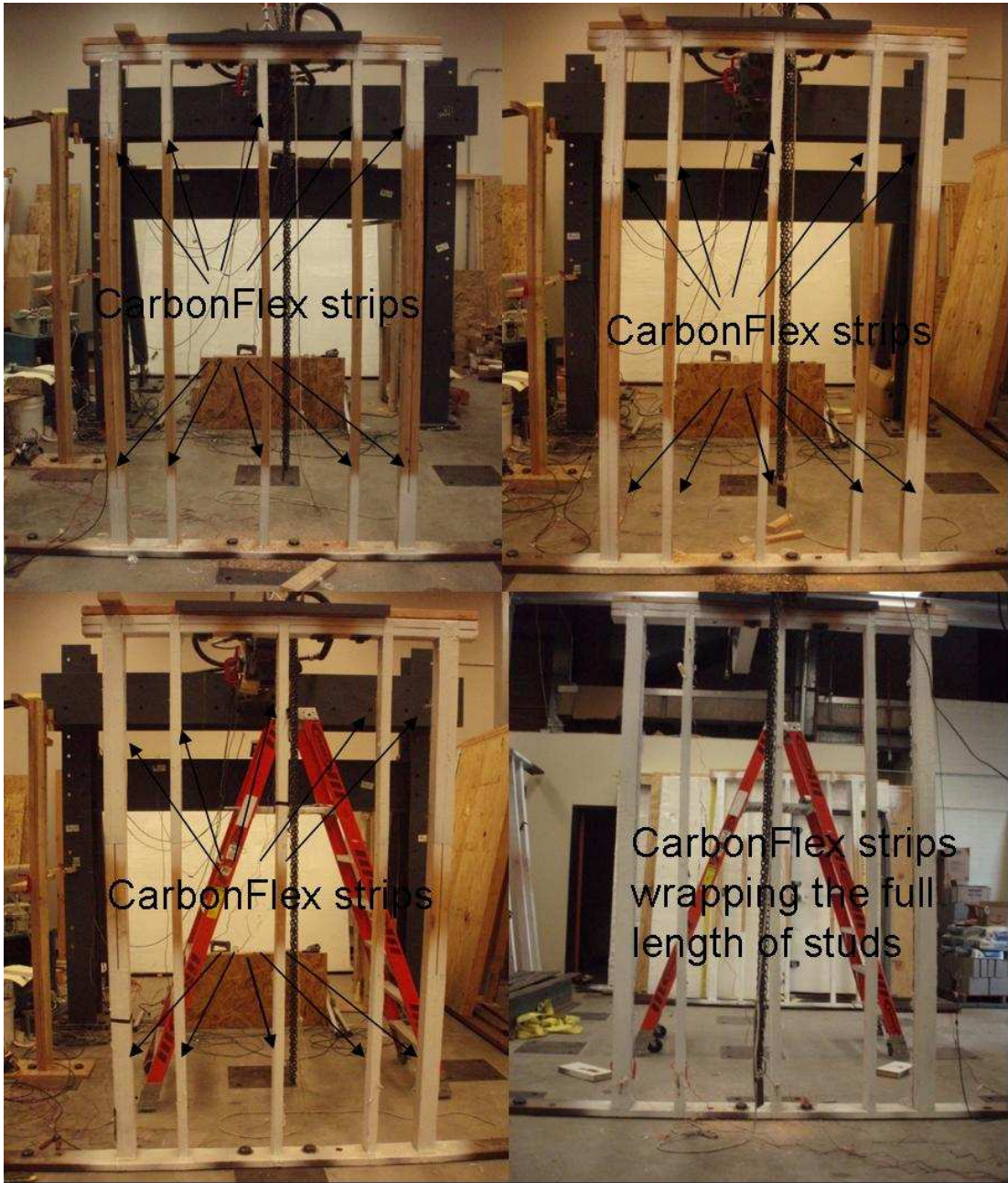
Figure 19. (a) 1 ft joint wrapped wall. (b) 2 ft joint wrapped wall. (c) 3 ft joint wrapped wall. (d) 4 ft joint wrapped wall.
