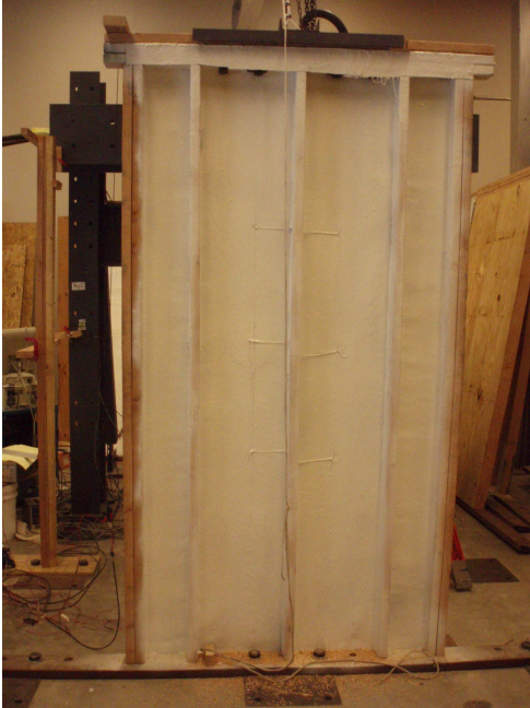
Figure 20. The CarbonFlex fully wrapped PPW wall.
