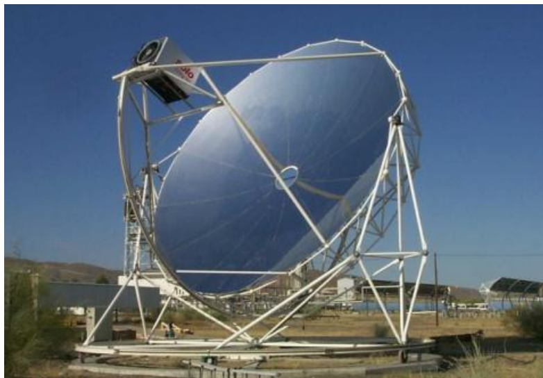
Fig 1.6 A Dish-Heat Engine System
