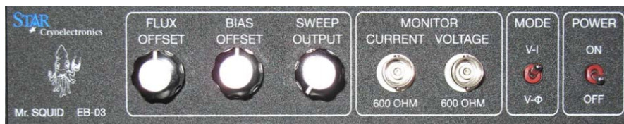
Figure 2.6. Picture of front panel of Mr. Squid box
