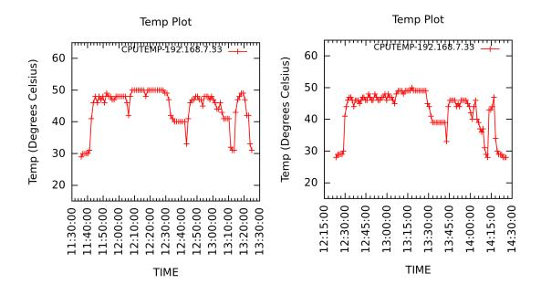
**Figure 5.27:** Temperature of Server 33 classified as "COLD" with FCFS(left) and TAS (right)
