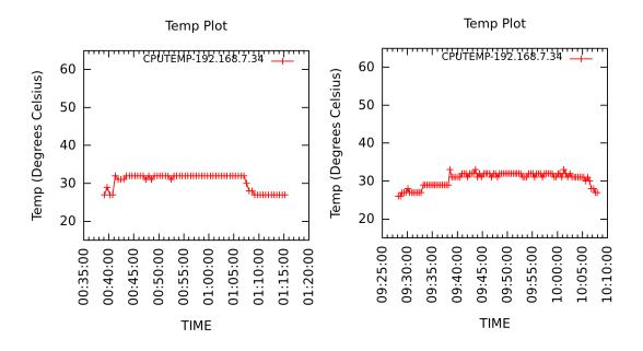
**Figure 5.46:** Temperature of Server 34 classified as "MEDIUM" with FCFS(left) and TAS (right)
