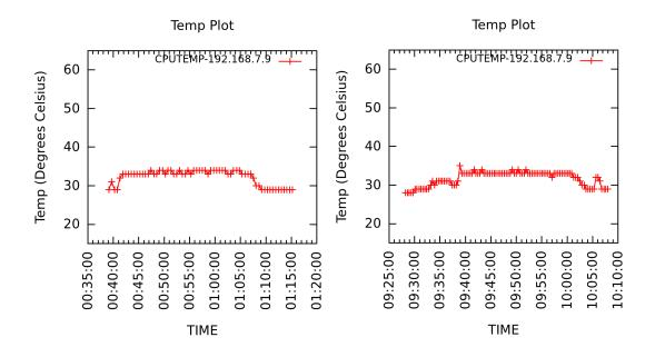
**Figure 5.44:** Temperature of Server 9 classified as "MEDIUM" with FCFS(left) and TAS (right)
