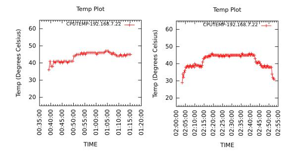
**Figure 5.32:** Temperature of Server 22 classified as "HOT" with FCFS(left) and TAS (right)
