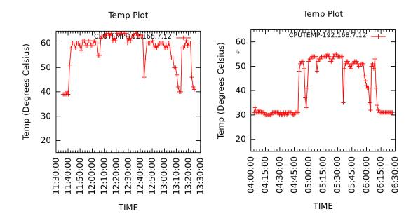
**Figure 5.7:** Temperature of Server 12 classified as "HOT" with FCFS(left) and TAS (right)
