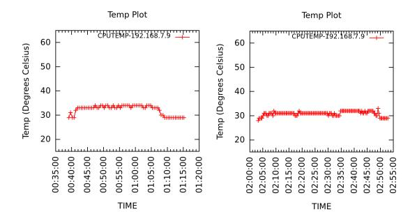
**Figure 5.33:** Temperature of Server 9 classified as "MEDIUM" with FCFS(left) and TAS (right)
