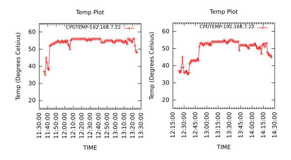
**Figure 5.20:** Temperature of Server 22 classified as "HOT" with FCFS(left) and TAS (right)
