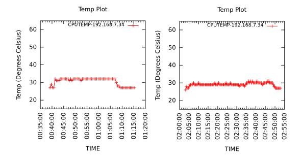
**Figure 5.35:** Temperature of Server 34 classified as "MEDIUM" with FCFS(left) and TAS (right)
