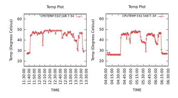
**Figure 5.12:** Temperature of Server 34 classified as "MEDIUM" with FCFS(left) and TAS (right)
