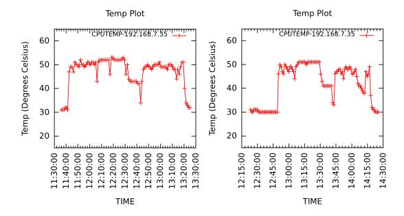
**Figure 5.19:** Temperature of Server 35 classified as "HOT" with FCFS(left) and TAS (right)
