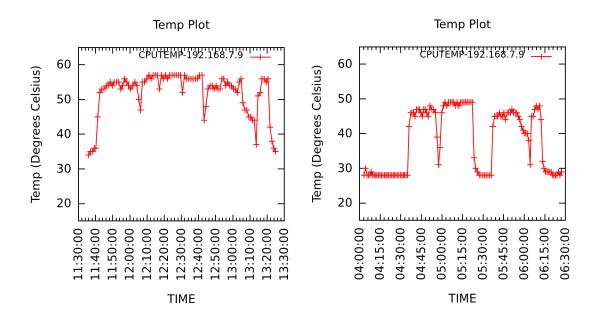
**Figure 5.10:** Temperature of Server 9 classified as "MEDIUM" with FCFS(left) and TAS (right)
