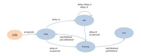
Figure 4.3: State Transition diagram of a TaskTracker.
