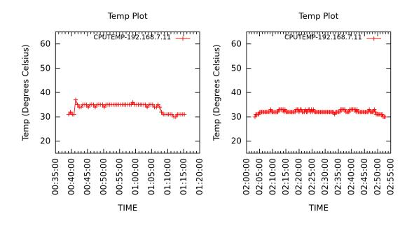
**Figure 5.29:** Temperature of Server 11 classified as "HOT" with FCFS(left) and TAS (right)
