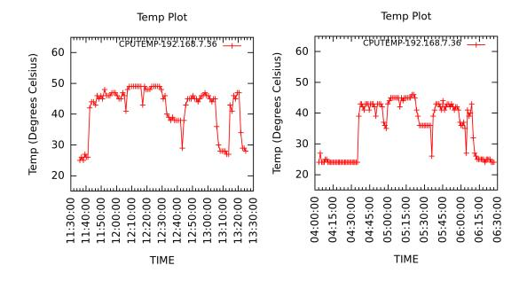
**Figure 5.13:** Temperature of Server 36 classified as "MEDIUM" with FCFS(left) and TAS (right)
