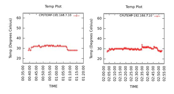
**Figure 5.34:** Temperature of Server 10 classified as "MEDIUM" with FCFS(left) and TAS (right)
