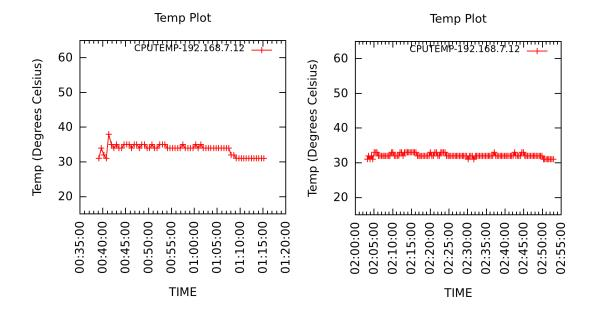
**Figure 5.30:** Temperature of Server 12 classified as "HOT" with FCFS(left) and TAS (right)
