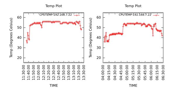
**Figure 5.9:** Temperature of Server 22 classified as "HOT" with FCFS(left) and TAS (right)
