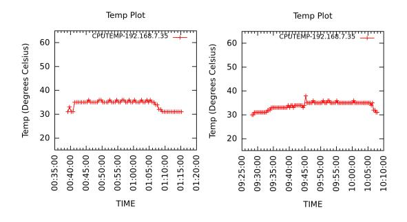
**Figure 5.42:** Temperature of Server 35 classified as "HOT" with FCFS(left) and TAS (right)
