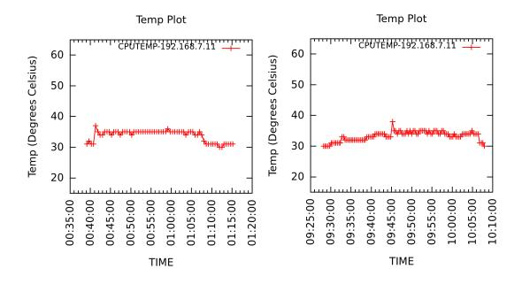
**Figure 5.40:** Temperature of Server 11 classified as "HOT" with FCFS(left) and TAS (right)
