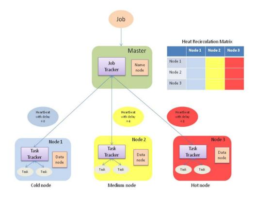
Figure 4.2: Overview of proposed scheme incorporating heat recirculation matrix
