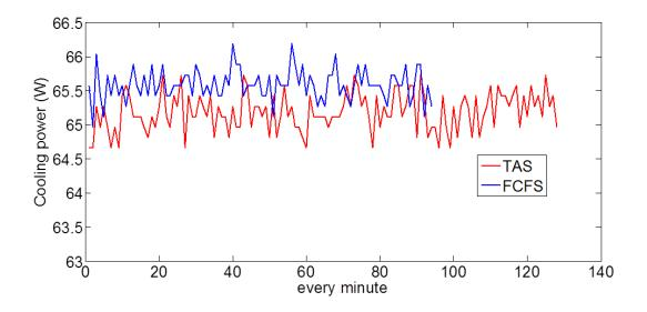
Figure 5.4: Cooling power for FCFS and TAS scheduler for PageRank workload with large delay
