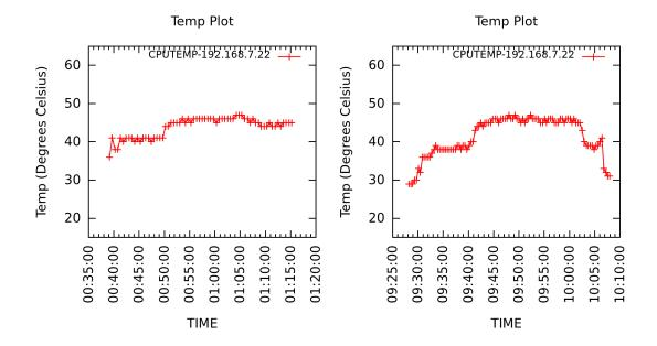
**Figure 5.43:** Temperature of Server 22 classified as "HOT" with FCFS(left) and TAS (right)
