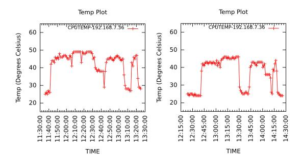
**Figure 5.24:** Temperature of Server 36 classified as "MEDIUM" with FCFS(left) and TAS (right)
