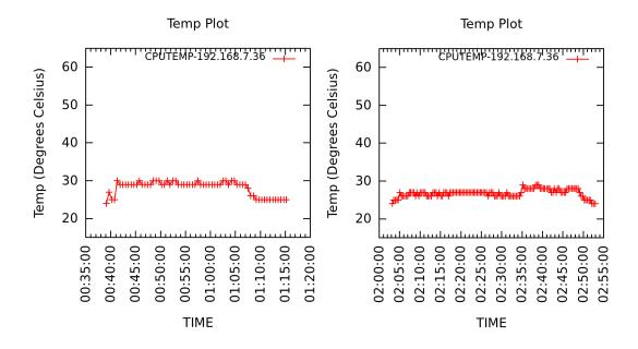
**Figure 5.36:** Temperature of Server 36 classified as "MEDIUM" with FCFS(left) and TAS (right)
