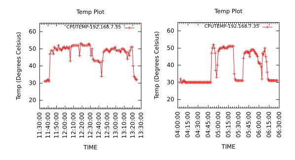
**Figure 5.8:** Temperature of Server 35 classified as "HOT" with FCFS(left) and TAS (right)
