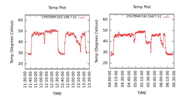
**Figure 5.14:** Temperature of Server 31 classified as "COLD" with FCFS(left) and TAS (right)
