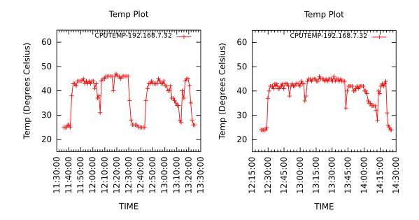
**Figure 5.26:** Temperature of Server 32 classified as "COLD" with FCFS(left) and TAS (right)
