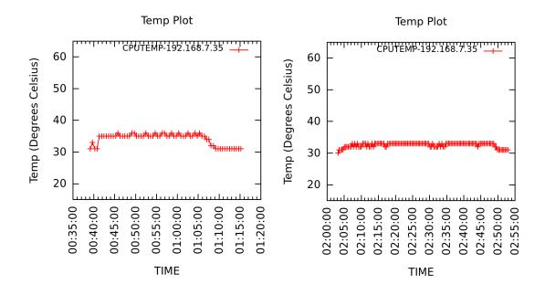
**Figure 5.31:** Temperature of Server 35 classified as "HOT" with FCFS(left) and TAS (right)
