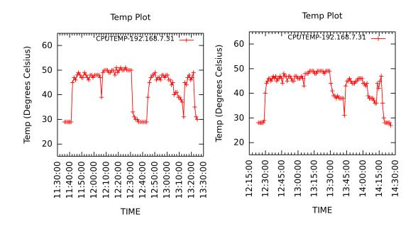
**Figure 5.25:** Temperature of Server 31 classified as "COLD" with FCFS(left) and TAS (right)
