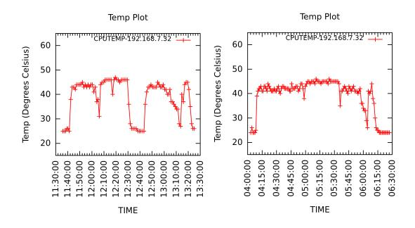
**Figure 5.15:** Temperature of Server 32 classified as "COLD" with FCFS(left) and TAS (right)
