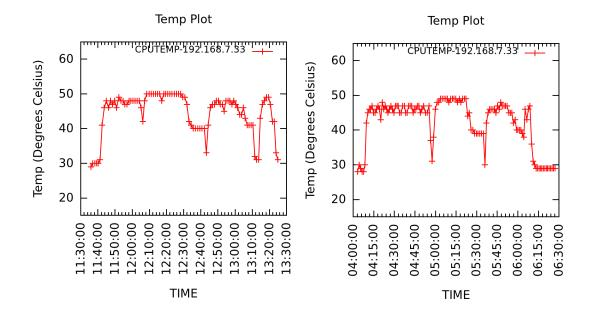
**Figure 5.16:** Temperature of Server 33 classified as "COLD" with FCFS(left) and TAS (right)
