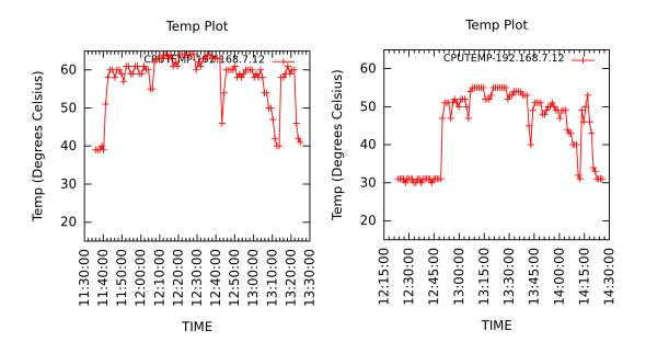
**Figure 5.18:** Temperature of Server 12 classified as "HOT" with FCFS(left) and TAS (right)
