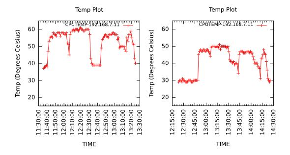
**Figure 5.17:** Temperature of Server 11 classified as "HOT" with FCFS(left) and TAS (right)
