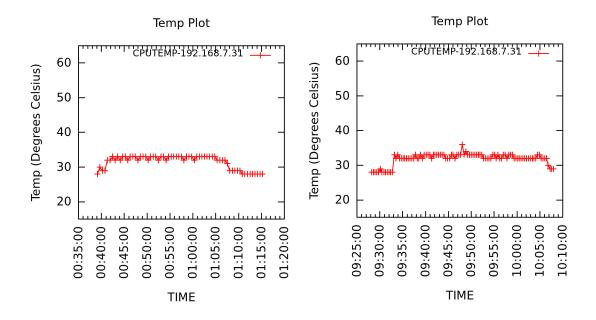
**Figure 5.48:** Temperature of Server 31 classified as "COLD" with FCFS(left) and TAS (right)
