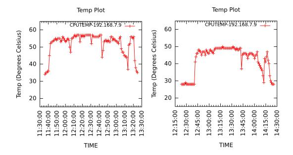
**Figure 5.21:** Temperature of Server 9 classified as "MEDIUM" with FCFS(left) and TAS (right)
