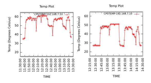
**Figure 5.22:** Temperature of Server 10 classified as "MEDIUM" with FCFS(left) and TAS (right)
