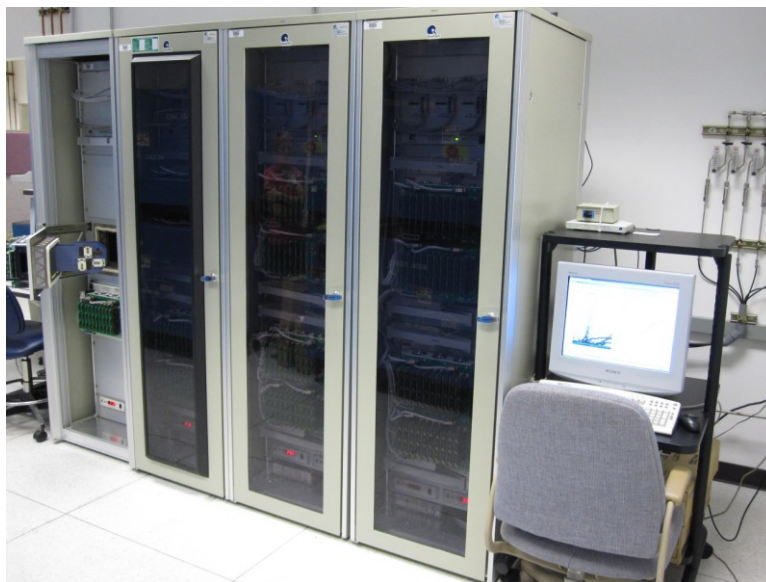
Figure 3.13 QualiTau MIRA electromigration test systems.
