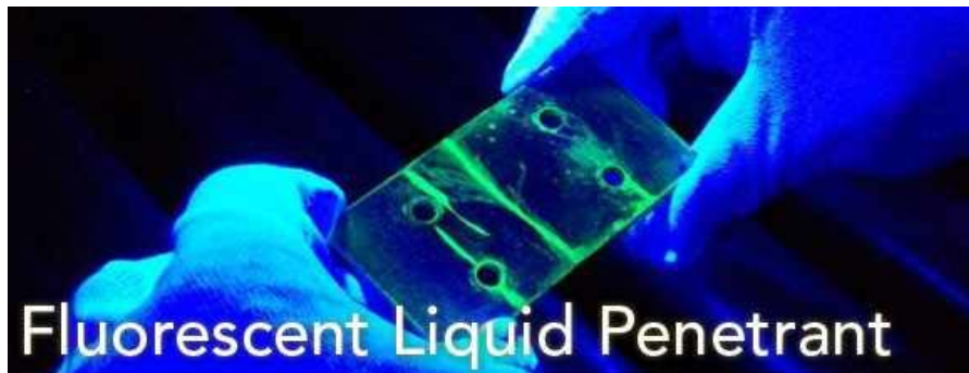
Figure 6: Fluorescent Liquid Penetrant applied to a part ( http://www.solaratm.com )
