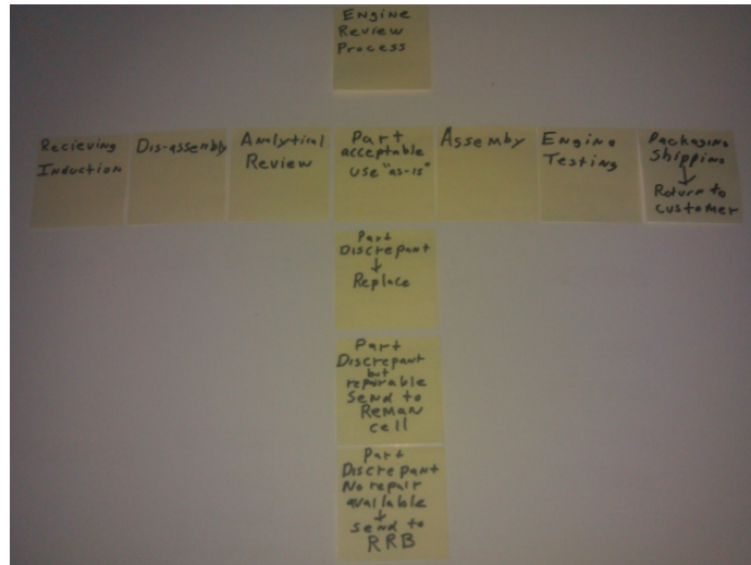
Figure 14: Initial process map of engine review process
