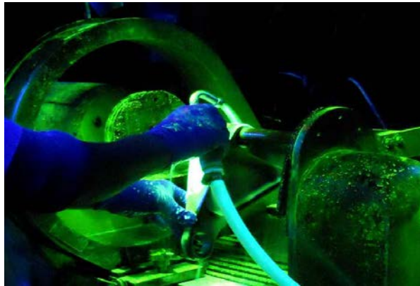
Figure 9: MPI technician applying the solution to component ( http://www.advancedcoatingtech.com )
