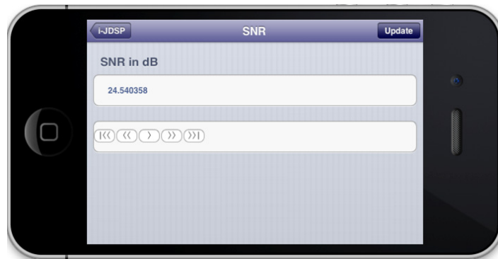
Figure 6.12: User interface of the SNR block. The SNR is displayed in decibels. The playback buttons allow traversal through the input frames to view the resulting SNR for each input frame.
