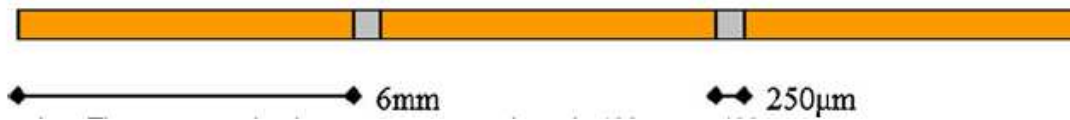
Figure 14: Sample configuration with three Cu segments and two SAC solder joints with 6 mm and 250 \mu\text{m} in length, respectively [21].
