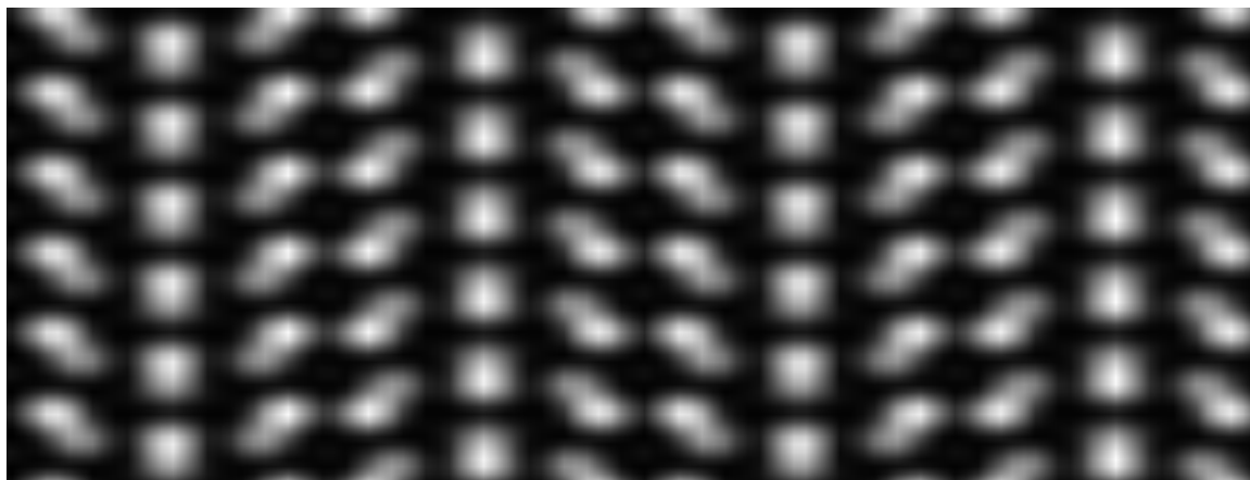
Fig (3.1.2.ii) STEMSLICE simulation of HAADF-STEM images for cross-sectional Cu(II)Se: dumbbells observed. Relatively bigger atom in the dumbbell is Se. Inclined dumbbells contain Cu Type A and Vertical (horizontal) dumbbells contain Cu Type B. Note that Cu type A and Cu type B actually end up closer together in this orientation. Simulation parameters: Projection = \langle 100 \rangle ; E_0 = 200\text{kV} ; C_s = 0.00\text{mm} ; df = 0.00 \text{ \AA}^0 ; Aperture = (0, 10.37) mrad; Size of \psi_{\text{probe}} : 256 x 256 pixels.
