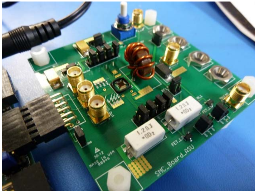
Fig. 42: Photo of Test PCB with Exposed Die (Courtesy of Space Micro).
