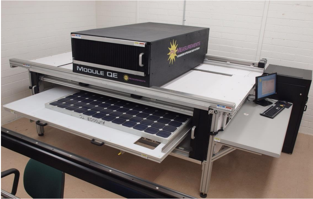
Figure 20. The Arizona State University Photovoltaic Reliability Laboratory Cell-Module Quantum Efficiency (C-M-QE) System
