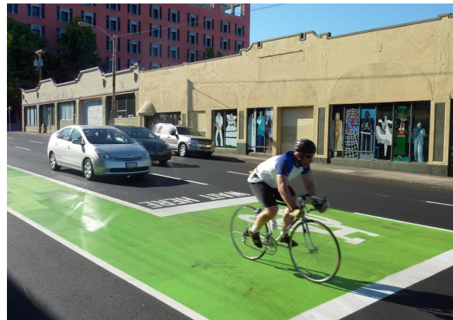
FIGURE 22. BICYCLE BOX, DEMARCATION THAT FEATURES A PAINTED AREA AT SIGNALIZED INTERSECTIONS FOR VISIBILITY OF BICYCLISTS
