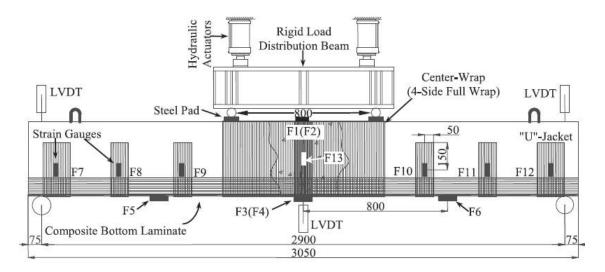
Figure 8. Retrofit schemes for CFRP retrofitting [5]
