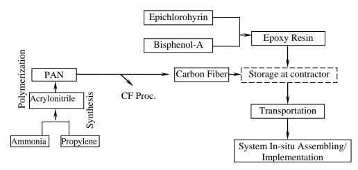
Figure 7. Elementary Flow of CFRP production (Cradle to Gate)
