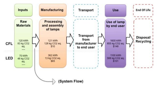
Figure 1: System Boundary used throughout the LCA
