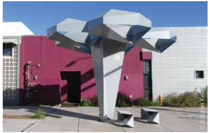
Figure 2 Tall sculptural features should leverage their height to provide shade, but designers should seek creative ways to shape its form to maximize shade area for multiple times of day. This example provides an identity feature for the neighborhood, but only provides shade on a few seats for a very short time around solar noon, when foot traffic in the area is lighter.
