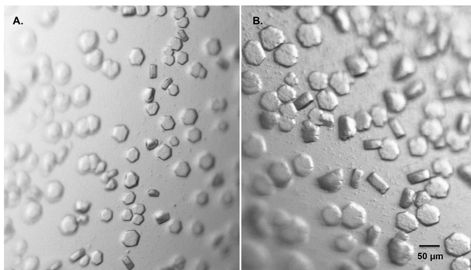
FIG. 3. Images of microcrystals prepared from virus at 1 mg/ml (a) and 4 mg/ml (b) of Sindbis virus prior to glutaraldehyde treatment. Samples A and B crystals exhibited sizes up to 25 \mu\text{m} and 50 \mu\text{m} , respectively. Scale bar = 50 \mu\text{m} .
