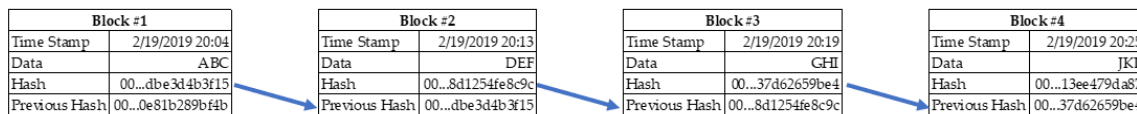
88 89 Figure 2. Creation of blocks of information: Every new block will have a timestamp, the data stored, the 90 previous and a new hash. The new hash is a function of all the information in the block. 91
