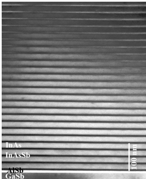
FIG. 2. Cross-section electron micrograph of sample G, demonstrating excellent structural quality.
