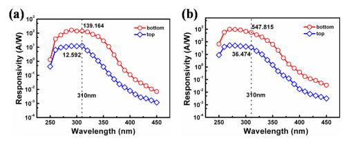
Fig. S2 The spectral response of (a) TUP and (b) TKP devices at 6V bias by applying the light from the top and the bottom.
