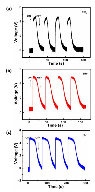
Fig. S4 The time response spectrum of the devices under periodic light pulses.
