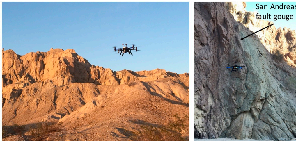
Figure 3. Example flight of a small unmanned aerial system (sUAS): in the Mecca Hills ( left ); and in Painted Canyon ( right ), acquiring low-altitude photos and to apply Structure from Motion along the San Andreas fault. The sUAS can image steep slopes to create topographic reconstructions with comparable horizontal and vertical resolution.
