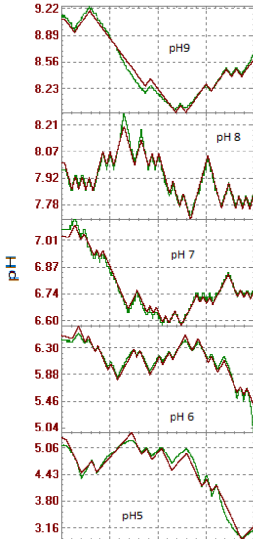
Figure 5, Open-loop Predictions of all models, -green actual output( y ) -red predicted output ( y_m )
